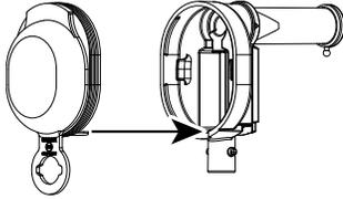
Wrap loop around lower opening to secure dome.
