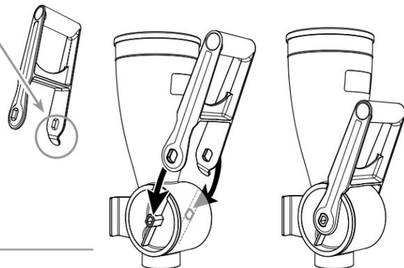
**4** ADD DISCHARGE FITTING TUBE to bottom opening of dispenser.
