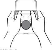
ASSEMBLE Press firmly to snap hinges together.
