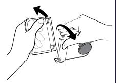
DISASSEMBLE Twist to snap hinges apart.
