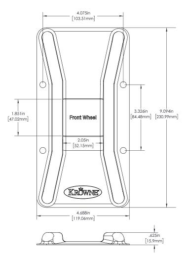
Krowne's Front Caster Positioning Chocks are designed to work with our 28-200 Rear Caster Chocks to meet local codes that require caster chocks on the front and rear wheels. Caster Chocks are designed to create a home position for all movable kitchen equipment to ensure they are always returned back to the proper location, in relation to fire suppression and ventilation systems after the removal for cleaning and maintenance purposes.
