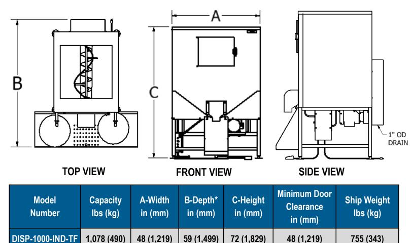
\*Depth includes 23" for the electrical components, ice chute, & shelf
