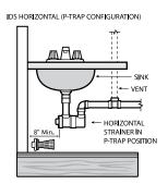
Unlike competitive products the body of the **Endura IDS** is supplied 'loose-assembled'. This means that when it comes to installation the installer retains the full benefit of being able to orientate the outlet to suit the installation, only solvent welding the main joint when the location and orientation have been confirmed. Be it a domestic or commercial application these four images show typical IDS installations.
