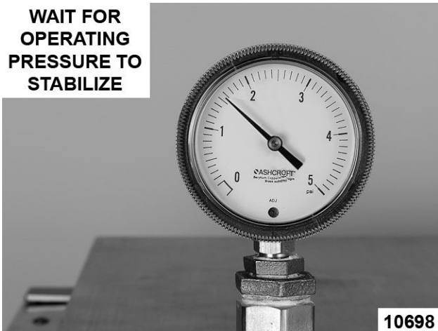
TYPICAL OPERATING PRESSURE
