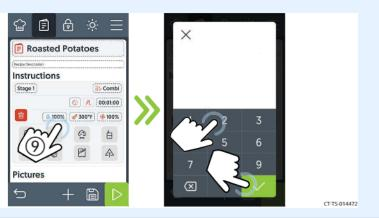
9. **Touch** the chamber temperature set-point icon ①. **Enter** the chamber temperature set-point using the key pad. **Touch** the check mark.
