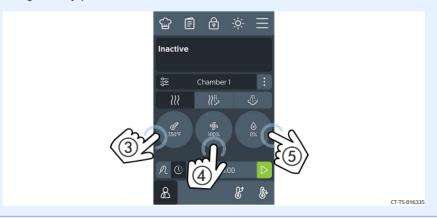
4. If cooking by time, **touch** the cook by time icon **(a)**. Then, **touch** the cooking time **(7)**. **Enter** the cooking time using the key pad. **Touch** the check mark.
