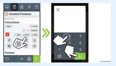
10. **Touch** the fan speed icon (1) to set the fan speed. **Touch** the check mark.
