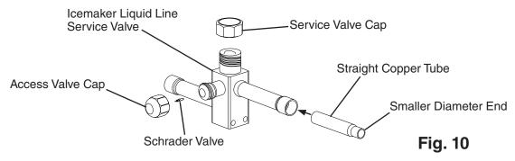
4) Braze the liquid line copper tube to the straight copper tube and the straight copper tube to the icemaker liquid line service valve.
