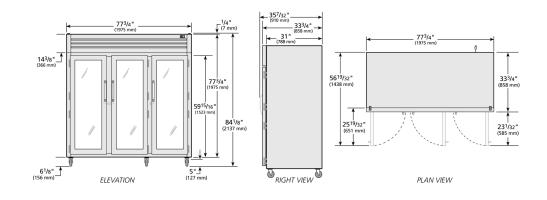
**SPECIFICATIONS** Dimensions 77¾ 1975 Depth 858 33¾ 1975 Height 77¾ U.S. Electrical International Horsepower 1/4 N/A Amps 6.1 Voltage 115/60/1 NEMA 5-15P Cord Length 9 ft. 2.74 M.
