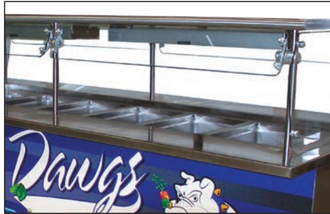
10-1/2" Standard Glass Opening (Maximum 13") From Table To Bottom Of Glass. NSF Requires Side Glass to be 18" Wide Minimum.
