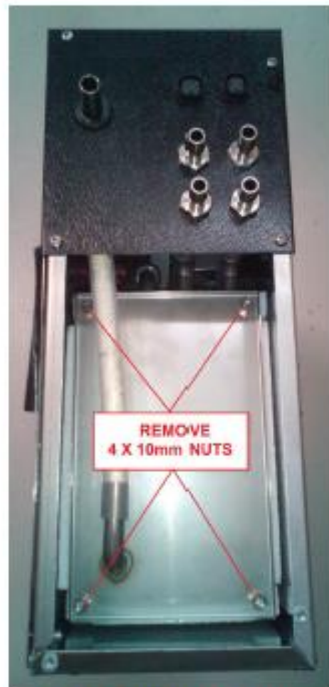
Figure 2. Water Tank Lid
